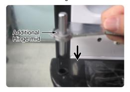
17. Assemble the assembled hinge and door to the refrigerator as below picture. Don't forget to insert washer with grease.
